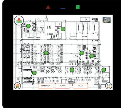
Gas detection layout on-site
